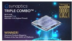
The Triple Combo SoC is the industry's first Matter-compliant solution that offers integrated Wi-Fi 6/6E, Bluetooth 5.2, and 802.15.4/Thread to enable a seamless wireless connectivity experience across multiple protocols, OEM brands, and platforms.
