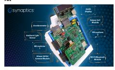
The Katana Edge AI EVK allows quick evaluation of the Katana low-power SoC and quick development of edge AI vision and sensor fusion applications.
